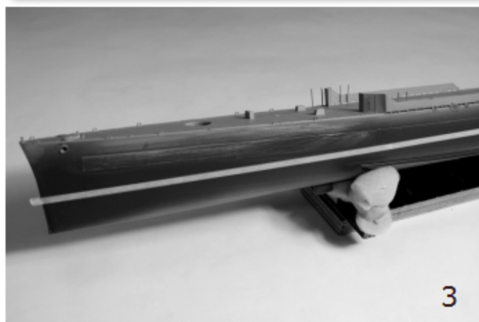
3 BLACK WATER LINE ZONE COVERED WITH MASKING TAPE .
