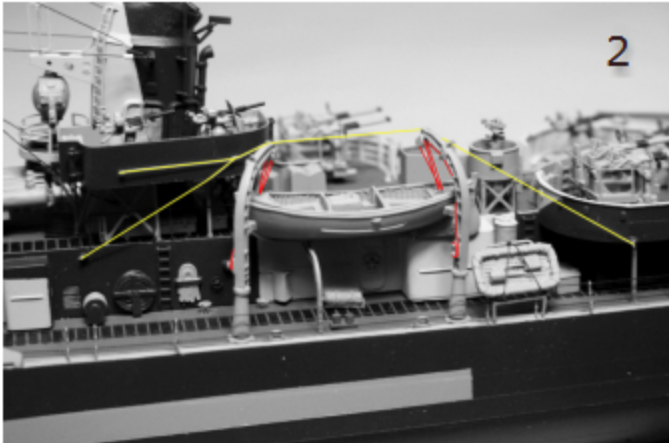
1, 2 MOTOR WHALEBOAT RIGGING. BOAT TACKLES ( RED ) AND JACKSTAY WITH FORE AND AFTER GUYS ( YELLOW ) ARE FROM LIGHT COLOR THREAD .
